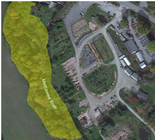
Figure 27. Vegetated buffer system (highlighted) preventing runoff to nearby river.
